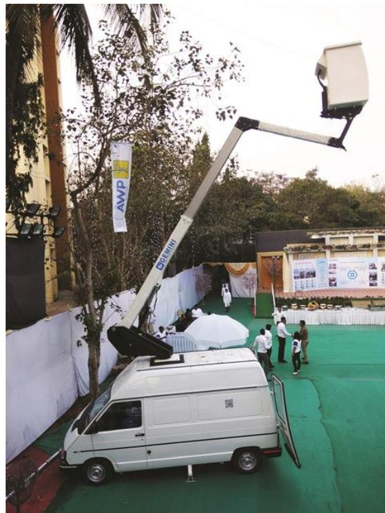
On the other hand, the truck mount, using Klubb’s 13m working height platform, is based on a 3.5 tonne GVW chassis and is also designed to be lighter and compact, compared to traditional truck mounts used in the market. “The chassis size reduces, and the width and the fuel reduces, the lane occupancy reduces. So, the TCO is reduced.
